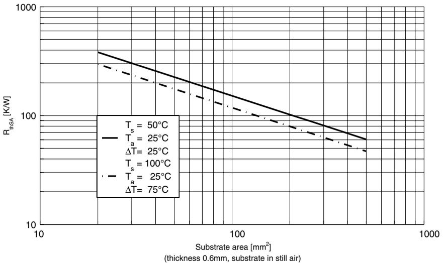
**Heat Dissipation from Al<sub>2</sub>O<sub>3</sub>-Substrate to Ambient Air**
