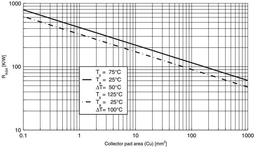
**Heat Dissipation from PC Board to Ambient Air**
