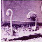
Equipment problems can also result in wire depression. For example, overcoat dispense tools that are improperly set up can land on the wires and depress them.
