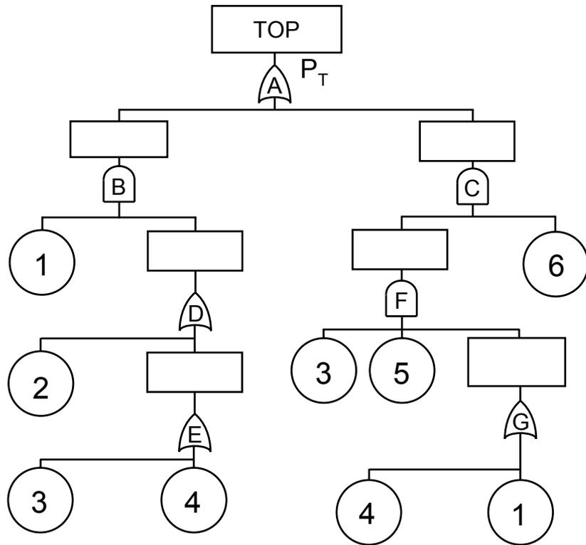
The quantitative importance of a Cut Set ( $I_k$ ) is the numerical probability that, given that TOP has occurred, that Cut Set has induced it.
