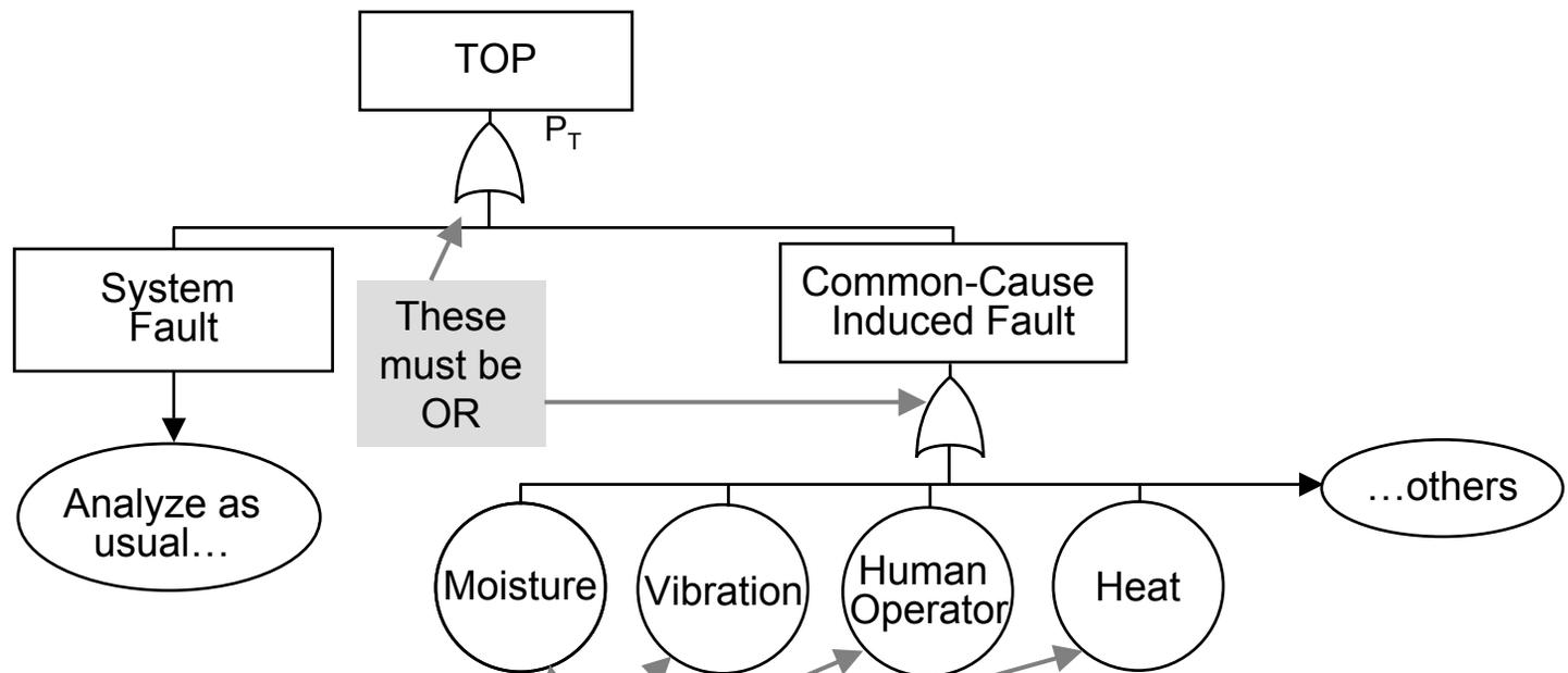
Introduce each Common Cause identified as a “Cut Set Killer” at its individual probability level of both (1) occurring, and (2) inducing all terms within the affected cut set.
