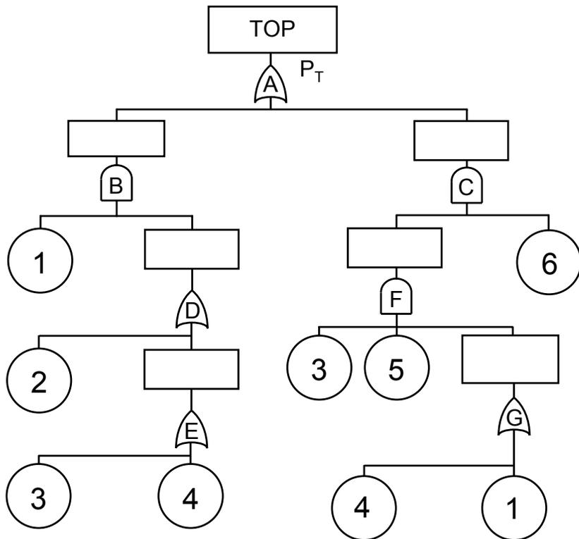
Cut Set Probability ( $P_k$ ), the product of probabilities for events within the Cut Set, is the probability that the Cut Set being considered will induce TOP.
