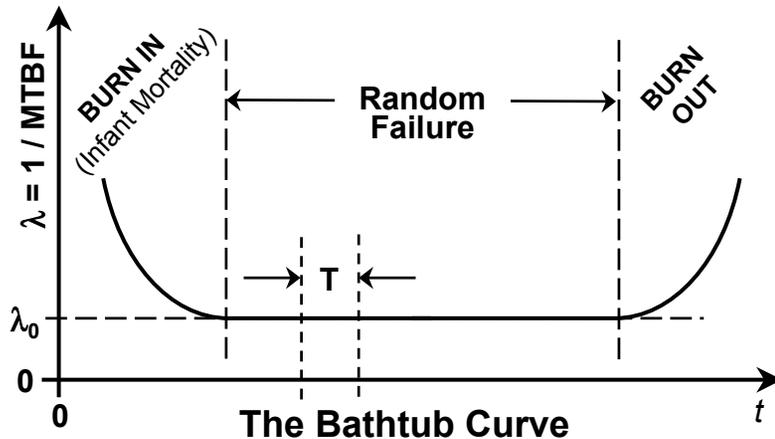
Most system elements have fault rates ( $\lambda = 1/\text{MTBF}$ ) that are constant ( $\lambda_0$ ) over long periods of useful life. During these periods, faults occur at random times.
