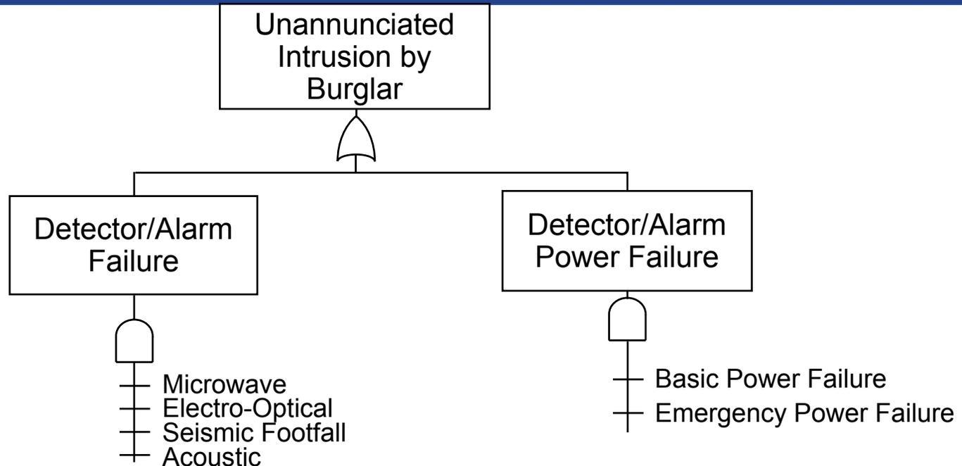
Here, power source failure has been recognized as an event which, if it occurs, will disable all four alarm systems. Power failure has been accounted for as a common cause event, leading to the TOP event through an OR gate. **OTHER COMMON CAUSES SHOULD ALSO BE SEARCHED FOR.**
