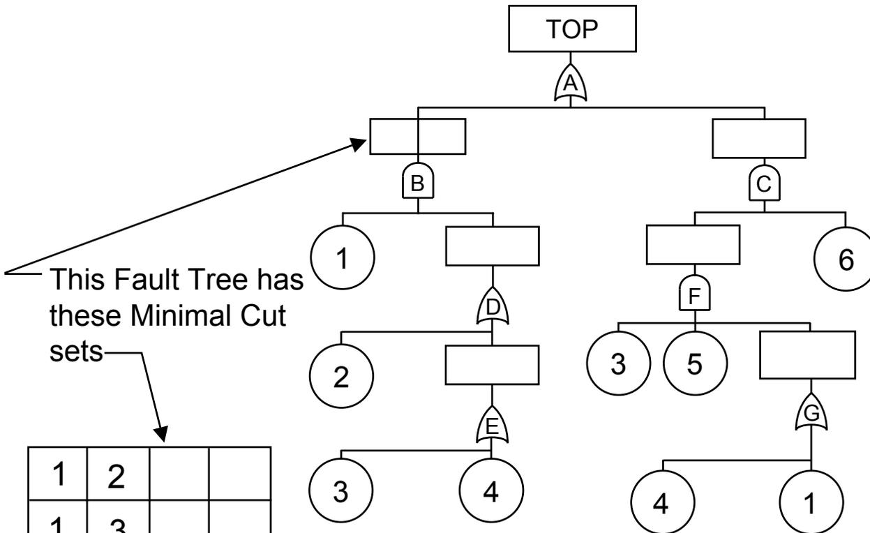
This Fault Tree has these Minimal Cut sets
