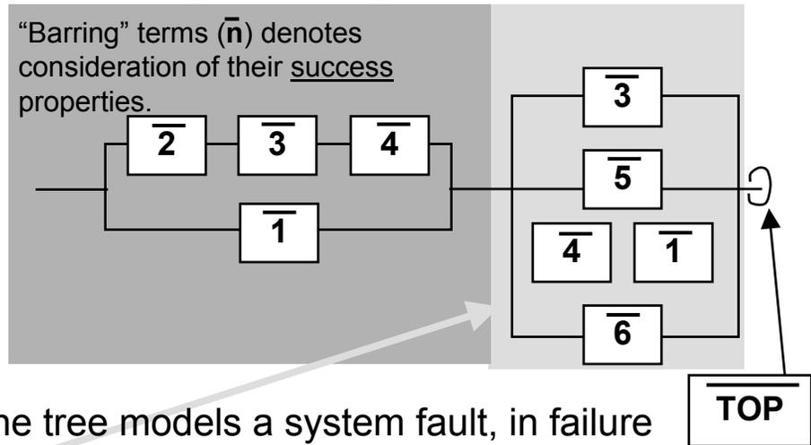
The tree models a system fault, in failure domain. Let that fault be **System Fails to Function as Intended**. Its opposite, **System Succeeds to function as intended**, can be represented by a Reliability Block Diagram in which success flows through system element functions from left to right. Any path through the block diagram, not interrupted by a fault of an element, results in system success.
