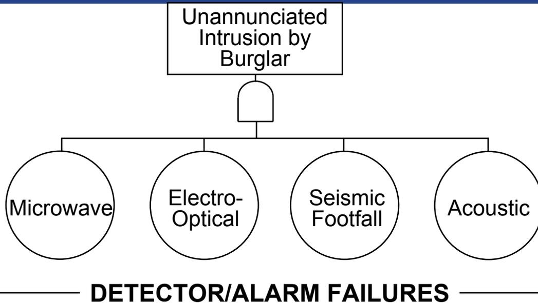
Four, wholly independent alarm systems are provided to detect and annunciate intrusion. No two of them share a common operating principle. Redundancy appears to be absolute. The AND gate to the TOP event seems appropriate. But, suppose the four systems share a single source of operating power, and that source fails, and there are no backup sources?
