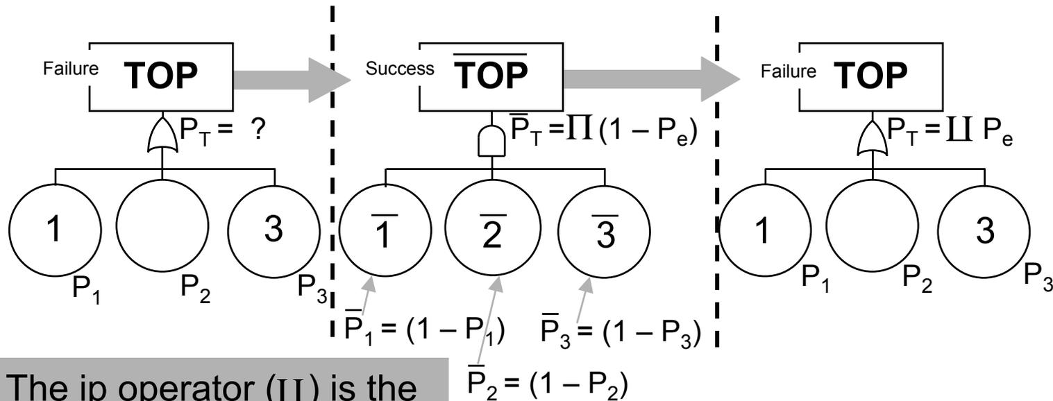
The ip operator ( $\coprod$ ) is the co-function of pi ( $\Pi$ ). It provides an exact solution for propagating probabilities through the **OR** gate. Its use is rarely justifiable.
