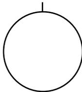
**Basic Event** – Initiating fault/failure, not developed further. (Called “Leaf,” “Initiator,” or “Basic.”) The Basic Event marks the limit of resolution of the analysis.
