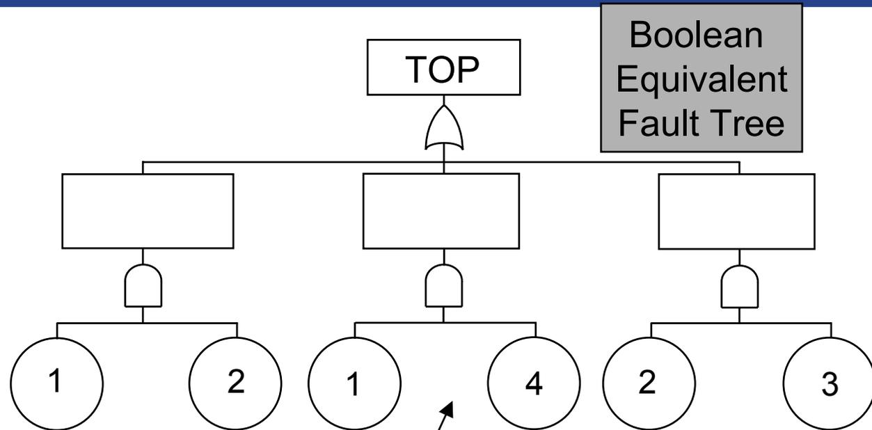
...and this Fault Tree is a Logic Equivalent of the original, for which the Minimal Cut Sets were derived.
