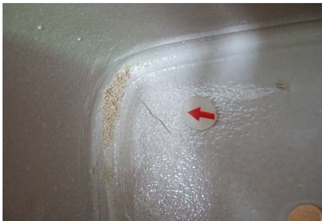
crack on tank
