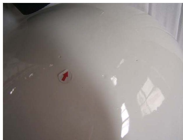
pin hole on seat-minor
